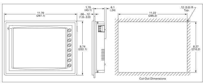
Figure 11. HMI10CE — Approximate Dimensions in Inches (mm)
